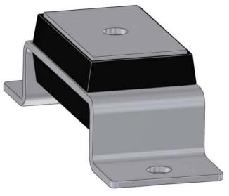
Many types of mechanical equipment cannot tolerate a high profile mount. CRM Mounts answer that need with a low profile, fail safe design. The all-directional captive rubber elements prevent metal to metal contact under normal use.
